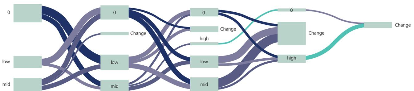
Results show a daily pattern of "mid-low-mid" engine temperature readings often appearing three days ahead of engine failure.
