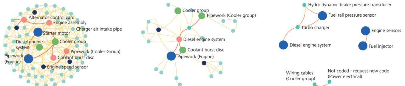
Nodes represent single repair codes. A line between nodes means that the two connected repair codes have appeared in the same train at least once (thicker lines mean more occurrences).
